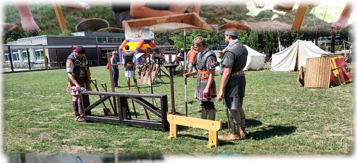
Small and large chorobates used as levels for the construction of aqueducts.
